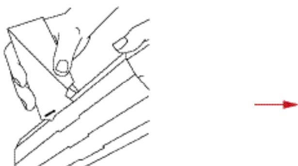
Insert the flaps of the elements into the slits in the central cylinder and cut off the ends on the inside.
